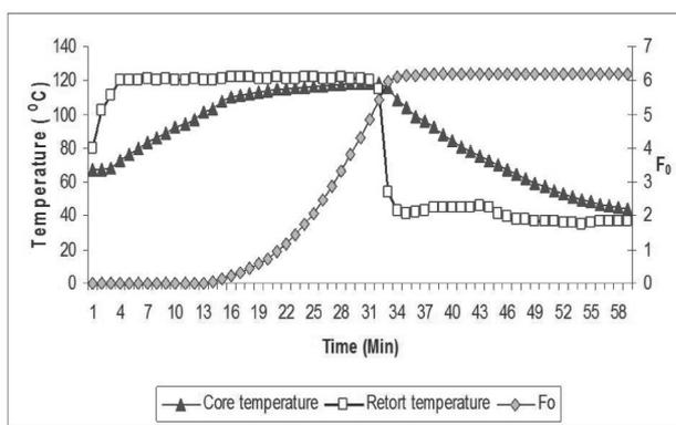
Fig. 3. Heat penetration characteristics with respect to  $F_0$  of crab koftha processed to  $F_0$  6 in TFS can
