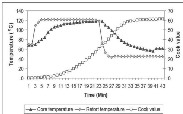
Fig. 2. Heat penetration characteristics with respect to cook value of crab koftha processed to  $F_0$  5 in TFS can
