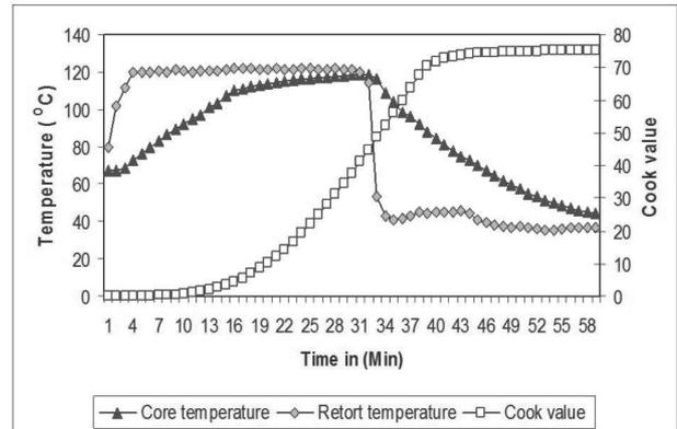
Fig. 4. Heat penetration characteristics with respect to cook value of crab koftha processed to  $F_0$  6 in TFS can
