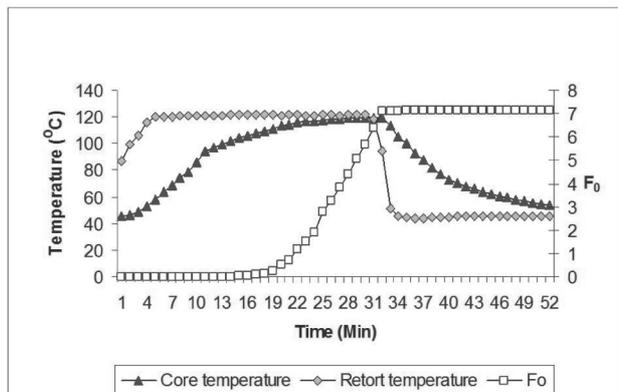
Fig. 5. Heat penetration characteristics with respect to  $F_0$  of crab koftha processed to  $F_0$  7 in TFS can
