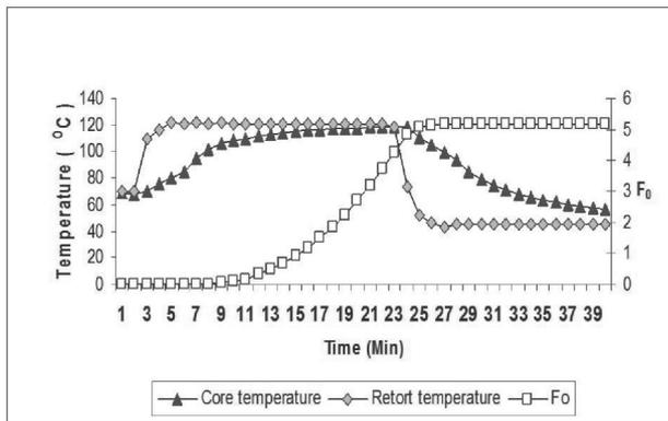
Fig. 1. Heat penetration characteristics with respect to  $F_0$  of crab koftha processed to  $F_0$  5 in TFS can
