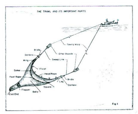
A typical trawl net and its important parts are indicated in Text Figure 1.
