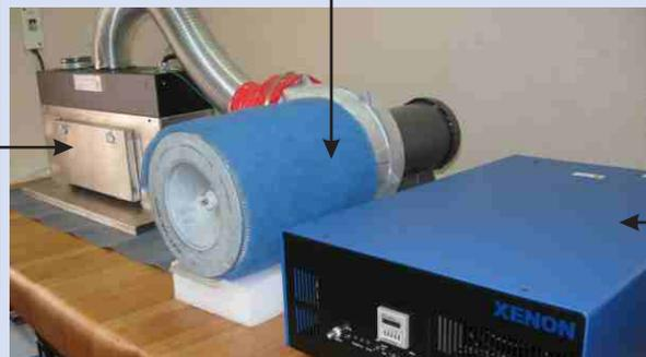
Pulse generator: Electrical energy is converted to short duration pulses of broad spectrum white light (200-1100 nm)
