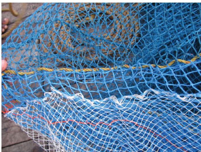
Square mesh codend covered with small mesh webbing (white) to retain escapes
