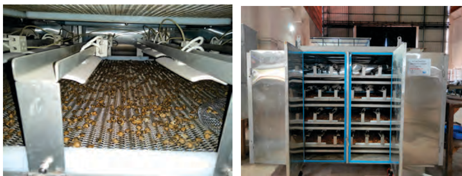
Clam drying process in pilot-scale hot air-assisted continuous infrared dryer
