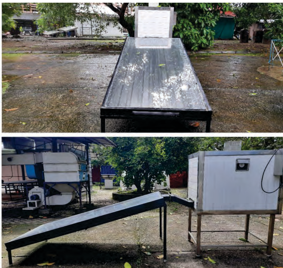
Solar-electrical hybrid dryer (10 kg capacity)
