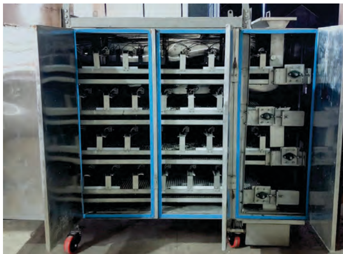
Pilot-scale hot air-assisted continuous infrared dryer for drying marinated anchovy
