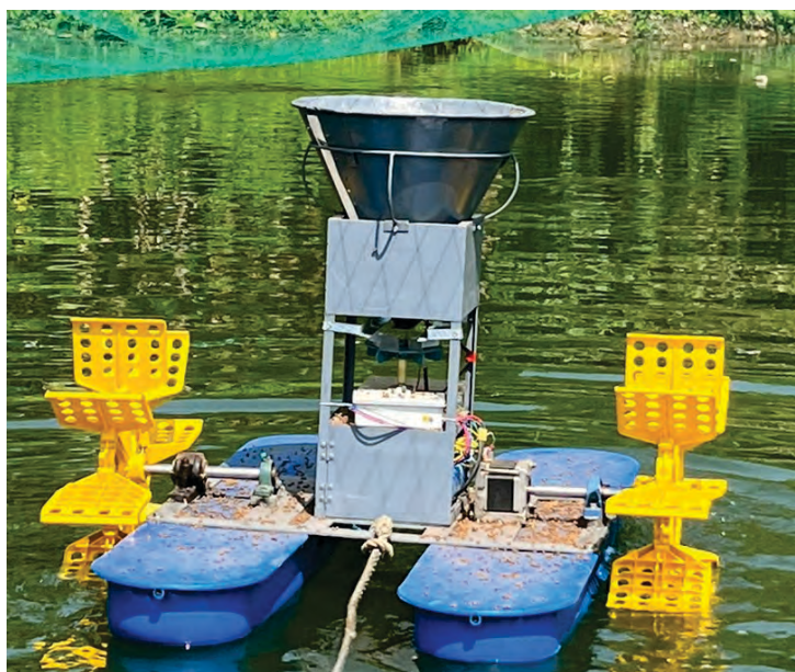
Improved design of solar-powered fish feed dispenser cum aerator
