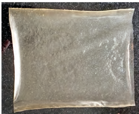
Chlorhexidine grafted Nanochitosan film
