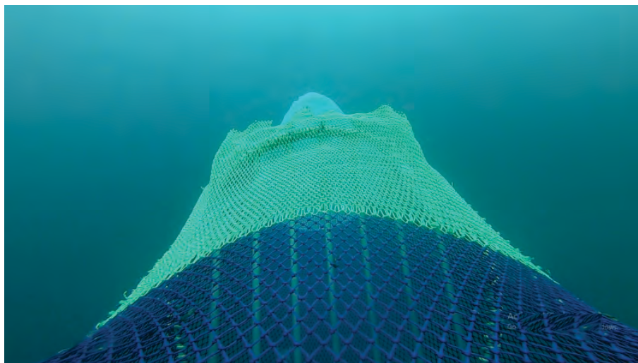
Underwater view of flap sealing of CIFT-TED captured on GoPro camera
