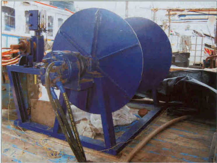
Fig. 3: Hydraulically driven indigenous monofilament longline spool
