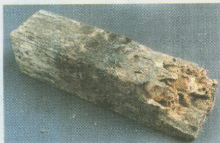
Soil burial test control panel
