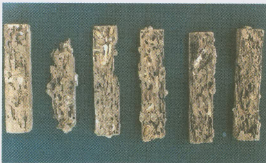
Untreated rubber wood panels exposed to sea water for 6 months
