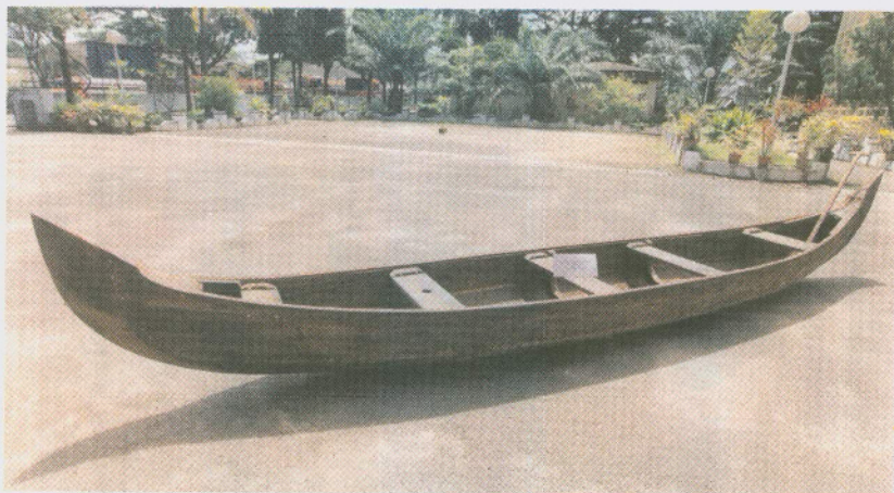
Treated rubber wood canoe
