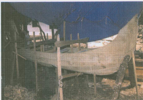
Rubber wood canoe under construction
