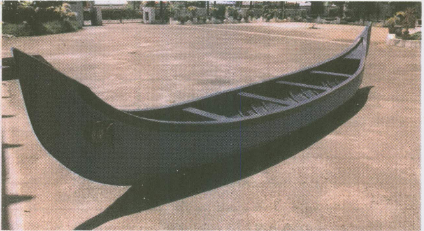
FRP sheathed rubber wood canoe
