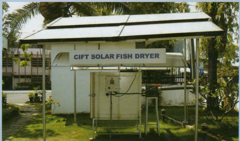
Solar dryer with electrical backup developed by CIFT, Cochin
