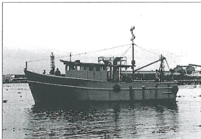
Fig. 3. MFV Sagarkripa - 15.5 m LOA, 120 hp fuel-efficient steel combination vessel
