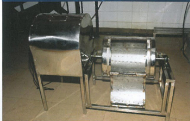
Fish de-scaling machine with fixed drum speed
