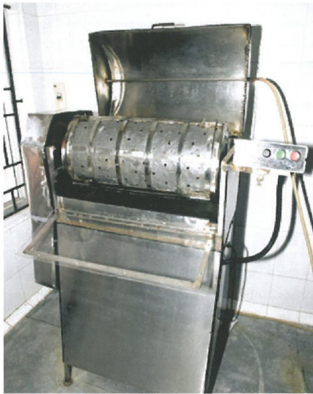
Fish de-scaling machine with variable drum speed
