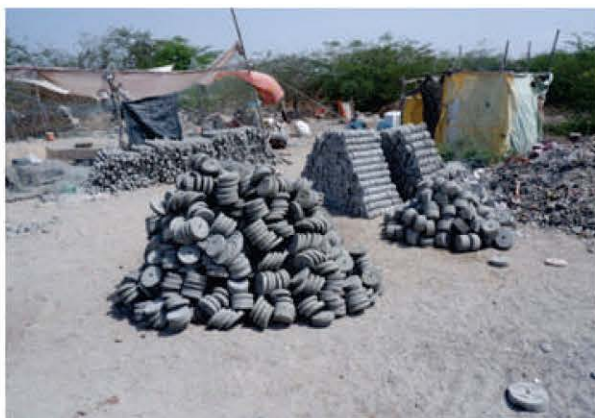
Various stages of fabrication of cement sinkers
