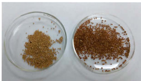
Fig 1. Chitosan silica bead (Bead 1) and chitosan alginate bead (Bead 2)
