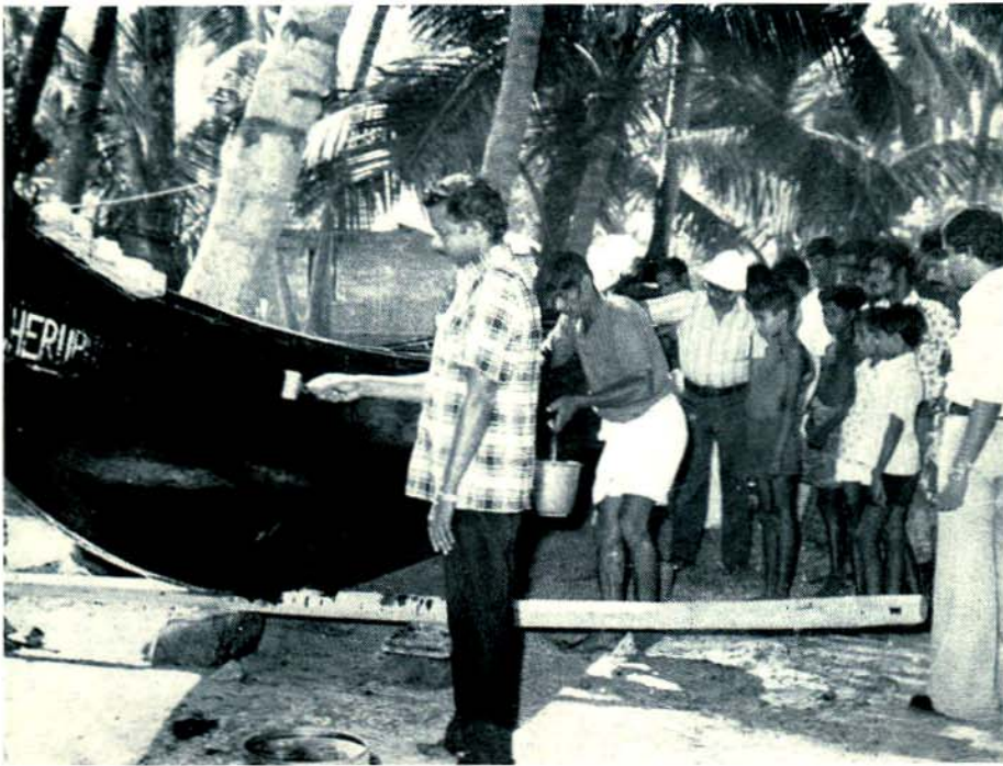
Application of a chemical preservative on an indigenous craft.
