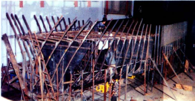
Construction of the 15.5 m. steel trawler of CIFT design in progress
