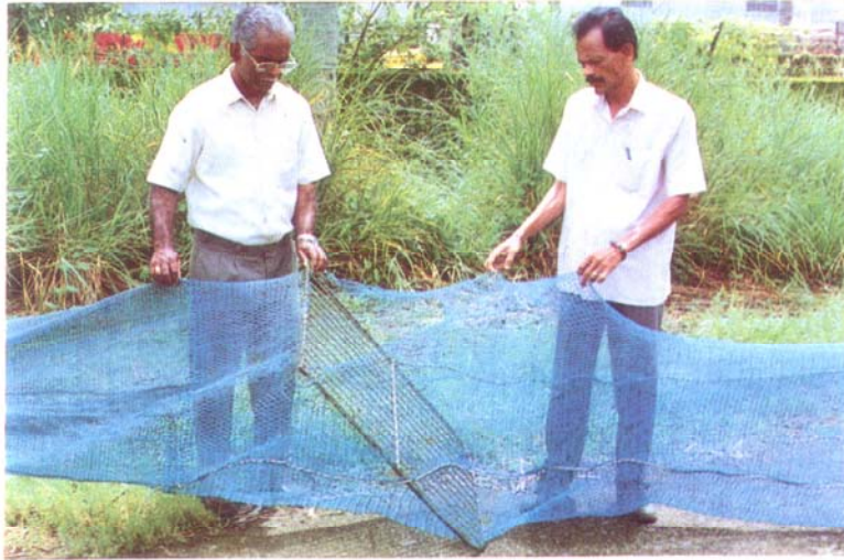
Selective device (grid with exit opening) fitted in the cod end of shrimp trawl for reduction of by-catch
