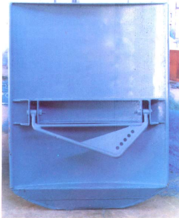
The 1350 x 1000 mm high aspect ratio suberkrub otter board designed for semi-pelagic trawling
