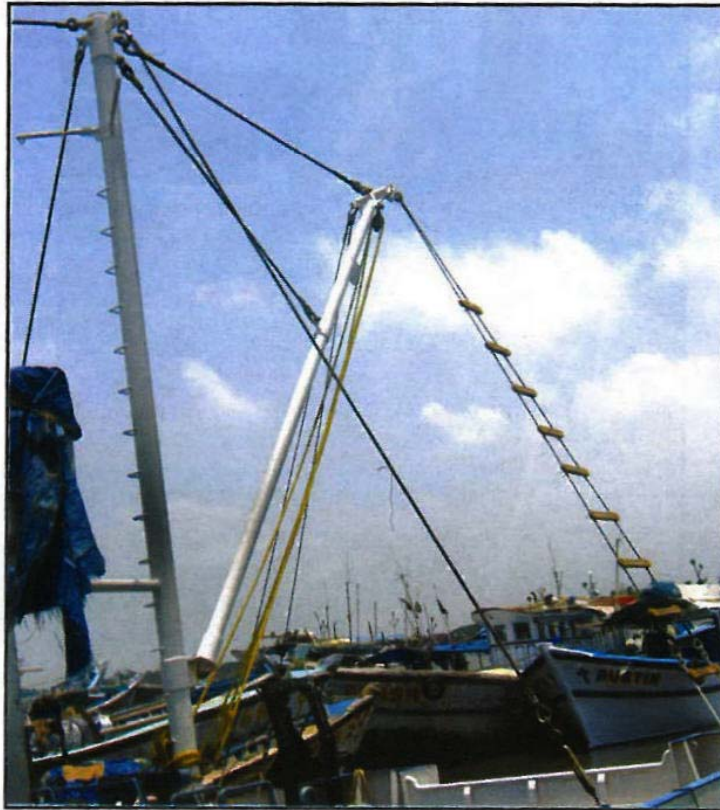
Fig. 14.3 Mast and boom arrangement in the aft deck of a small trawler
