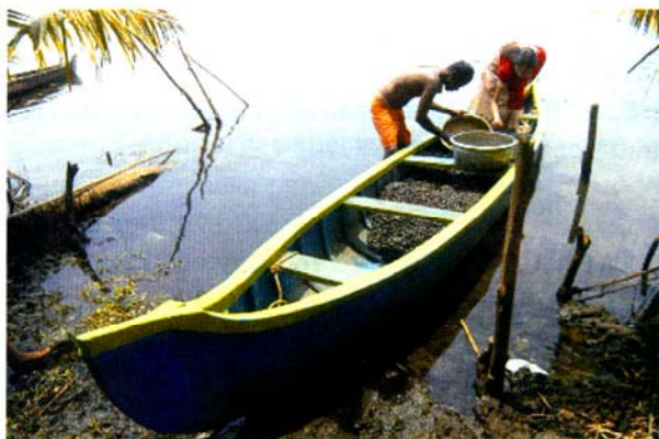
FRP sheathed rubber wood canoe for artisanal sector
