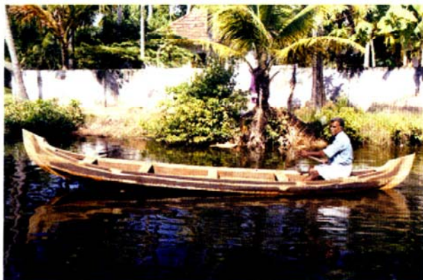
Dual preservative treated rubber wood canoe
