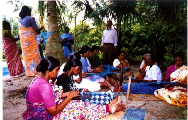
Fabrication of square mesh cod end
