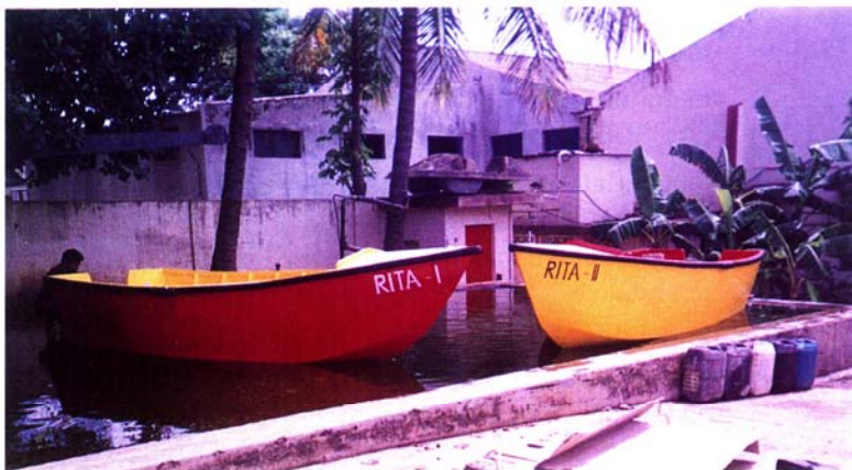
4.75m OAL flat bottom FRP boats designed and constructed for Burla Centre
