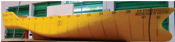
Fig. 2. Model of the 19.75 m multipurpose fishing vessel used for testing at IIT Chennai
