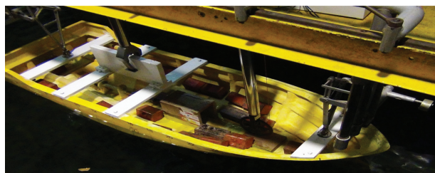
Fig. 3. Model test progressing in the towing tank at IIT Chennai
