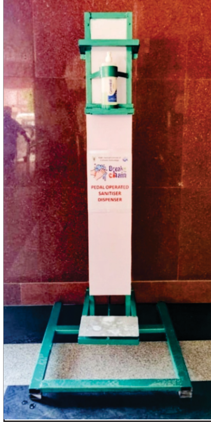
Stand-alone pedal operated hand sanitizer unit developed at ICAR-CIFT
