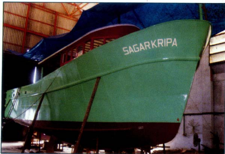
The 15.5 m fuel efficient steel trawler
