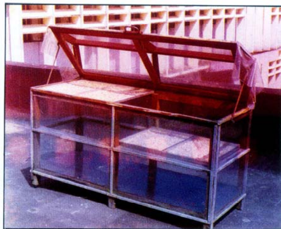
The 10 kg capacity PVC solar drier
