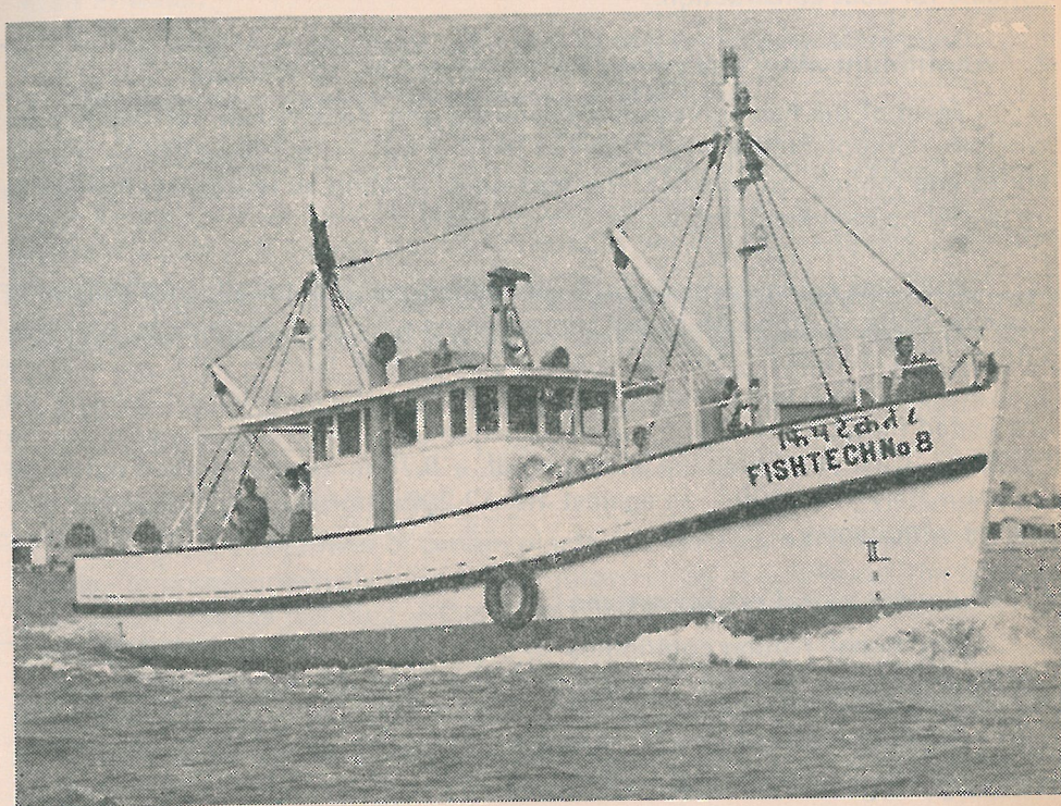
15 m. mechanised wooden fishing boat-designed and built at CIFT
