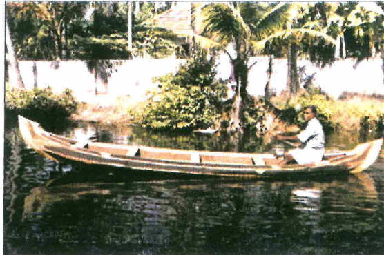
Dual preservative treated rubber wood canoe for traditional sector
