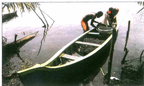
FRP sheathed rubber wood canoe for artisanal sector
