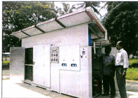
Solar dryer with LPG back-up
