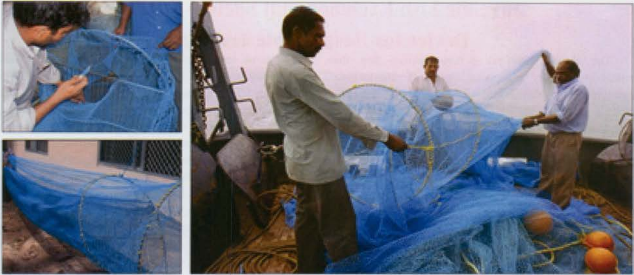
Fig. 2. Views of JFE-SSD under fabrication (upper left), ready for installation (lower left) and its operation (right)
