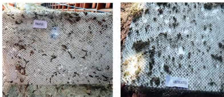
Treated and untreated cage webbings after seven months
