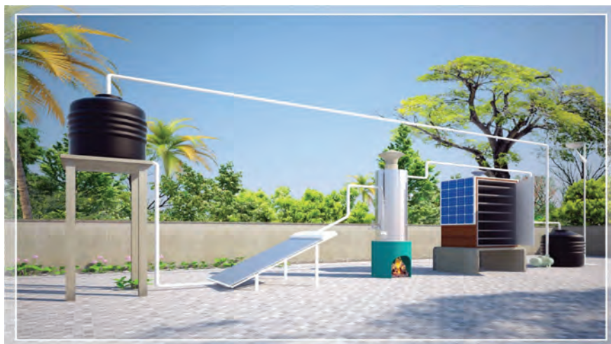
3D diagram of proposed multipurpose solar thermal conversion system with biomass heater backup
