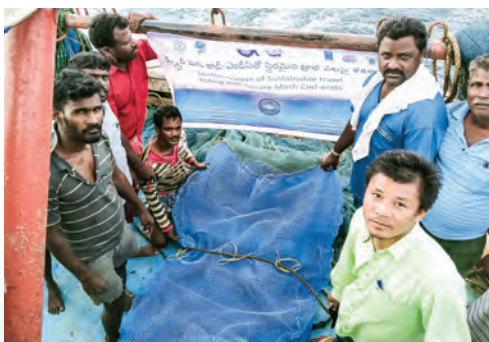
Onboard demonstration of square mesh cod end
