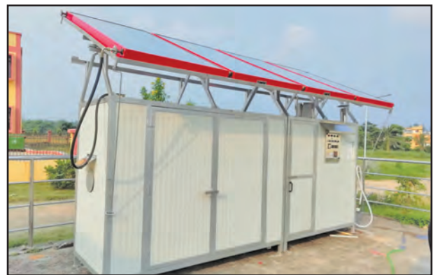
Solar Dryer established at ICAR-CIWA, Bhubaneswar, Odisha
