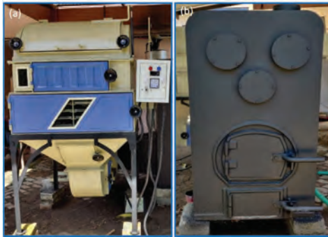
Low emission biomass dryer with drying chamber (a) and Biomass furnace (b)
