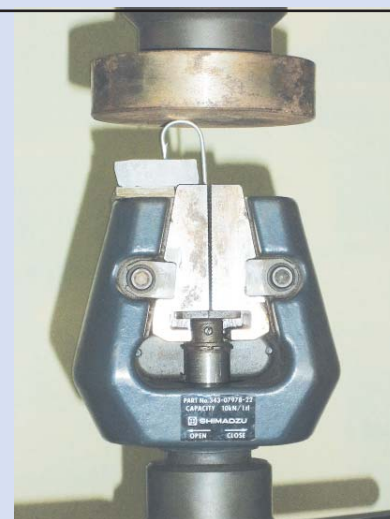
Experimental setup showing sharpness test using Universal Testing Machine
