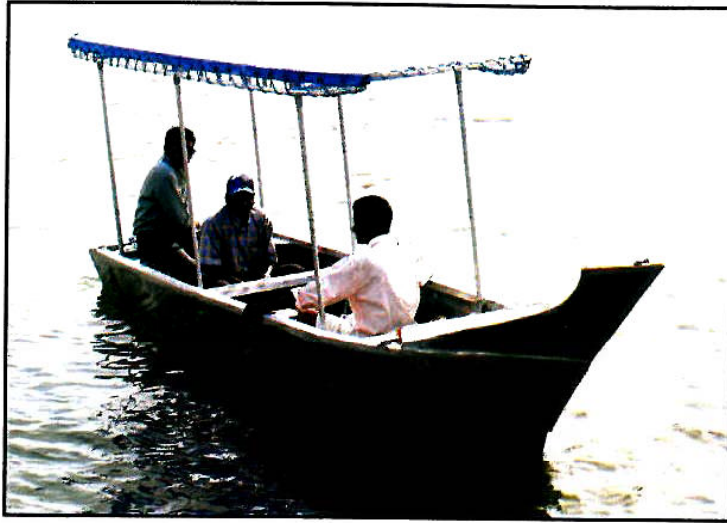
Fig. 4.4 Aluminium craft (5.2 m L_{OA} ) for inland fishing
