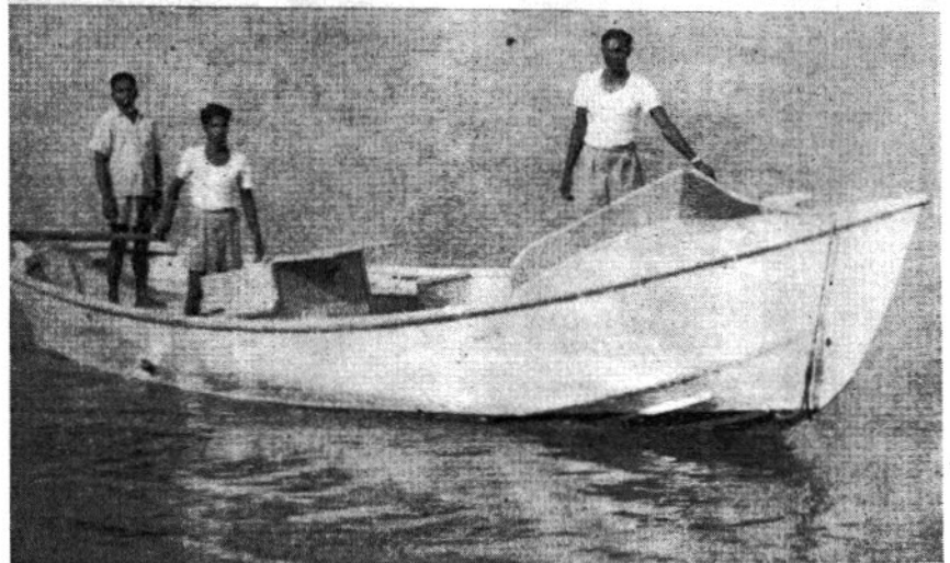
Completed sheathing, the two layers of FRP undergoing post curing. Further surface preparation and pointing procedures are being chalked out (top). A 25' open type beach-boat made of marine plywood and Fibre glass sheathing (FISH TECH No. 3, CIFT, Cochin)
