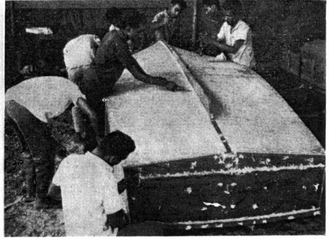
Measuring the area of the wooden hull to be sheathed with FRP. (Left). Filling up bolt holes, seams, crevices and corners with special seaming compound, and surface preparation
